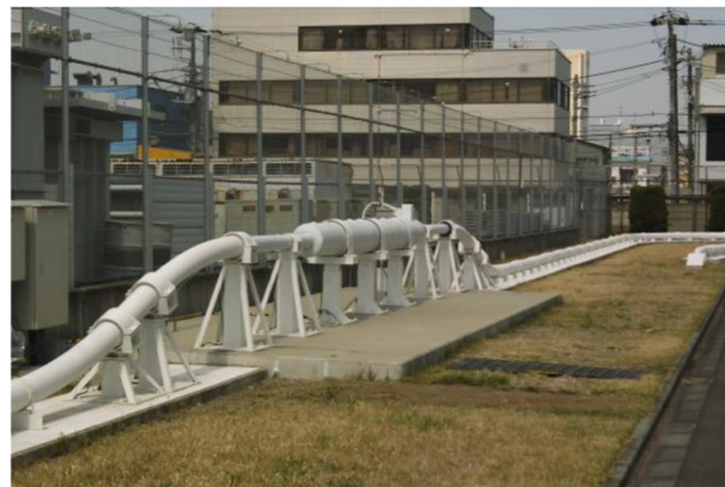
Fig. 2. TEPCO/Sumitomo 66 kV AC HTS test station at Asahi substation in Yokohama/Japan: left image shows the cable with a joint, right image shows the 66 kV AC end stations responsible for the transition from standard conductor to superconductor and from room to cryogenic temperature (2014).
