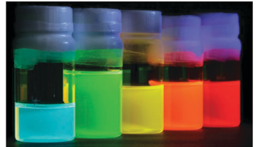
Colloidal CdSe nanocrystals (NC), diameter 1.7-4.5 nm (left to right) under UV illumination.
