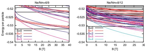
Fig. 3. Spectra of homogeneous systems with six and eight particles ( $\nu = \frac{2}{3}$ ) with Zeeman splitting displayed as a function of magnetic field. There is a direct crossing between the unpolarized ( $S = 0$ ; horizontal line) and fully polarized ( $S = 3$  and 4 for six and eight particles, respectively; the steepest line) state, i.e.  $B_c \approx 13$  and 8 T for six and eight particles, respectively. The crossing states are separated from the quasicontinuum by a finite gap.
