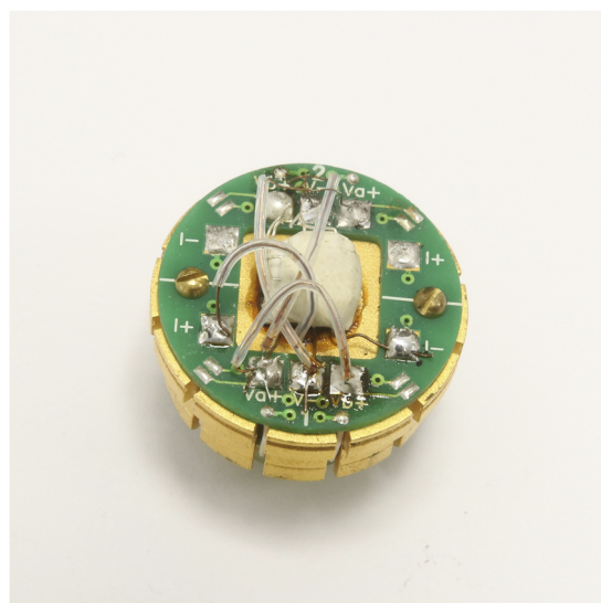
FIG. 4. Resistivity sample puck with the installed Hall sensor.
